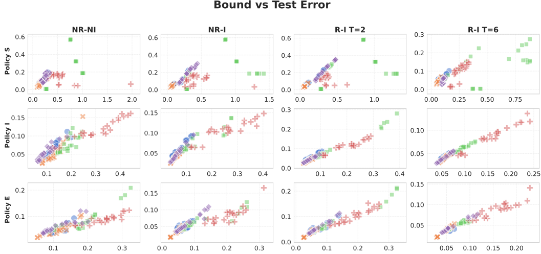
Figure 2: Correlation plots. PAC-Bayes bounds, one in each column, are plotted on the x-axis against true test errors on the y-axis for each method across all environments, policy instances, and repetitions to visualize correlation. Environments are color-coded as follows: Ant (blue circle), Half-Cheetah (orange cross), Hopper (green square), Humanoid (red plus), and Walker2d (purple diamond).
